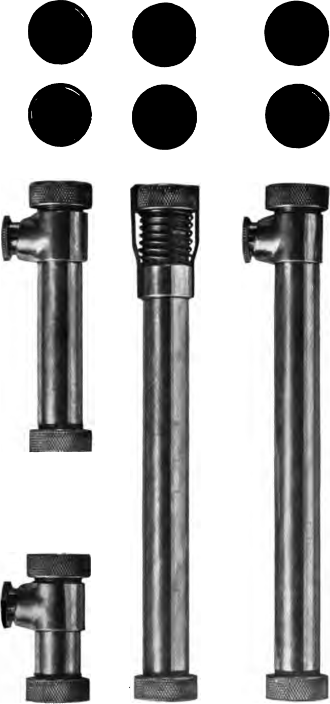
TUBES AND DISKS FOR DETERMINING COLOR OF WATER.
