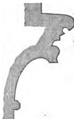
CAP OF TOWER ARCH.
