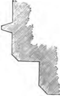
SECTION OF HEAD OF TRANSEPT DOORWAY: EXTERIOR.
