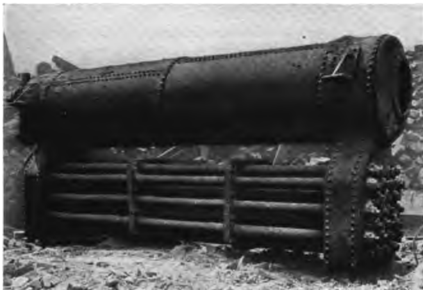
The First Heine Boiler, Built in 1882. Still Good for High Pressure after Thirty-five Years of Continuous Service.
