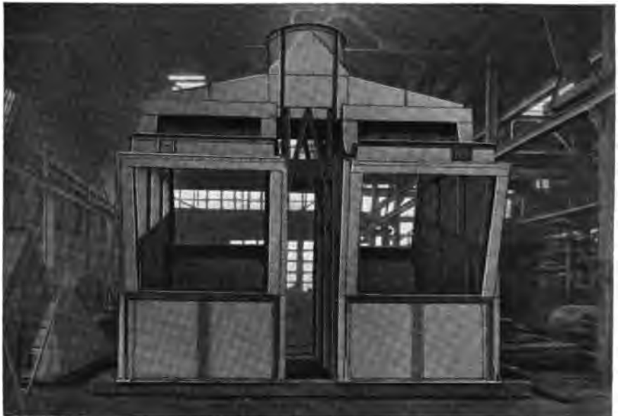
Rear View of Marine Casings for a Battery of Two Heine Cross Drum Marine Boilers.
