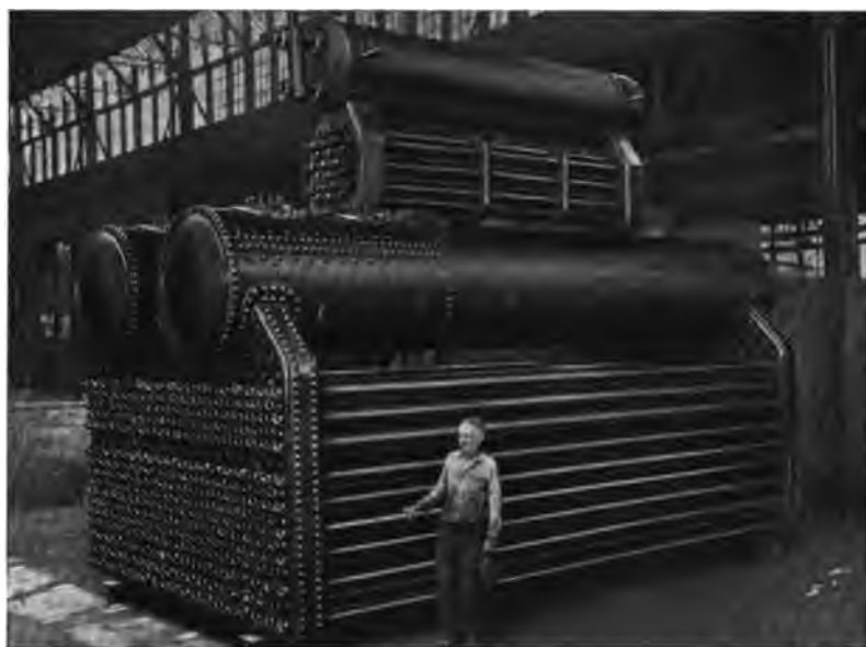
Comparative Sizes of the First Heine Boiler and a Standard 500 H. P. Boiler.
