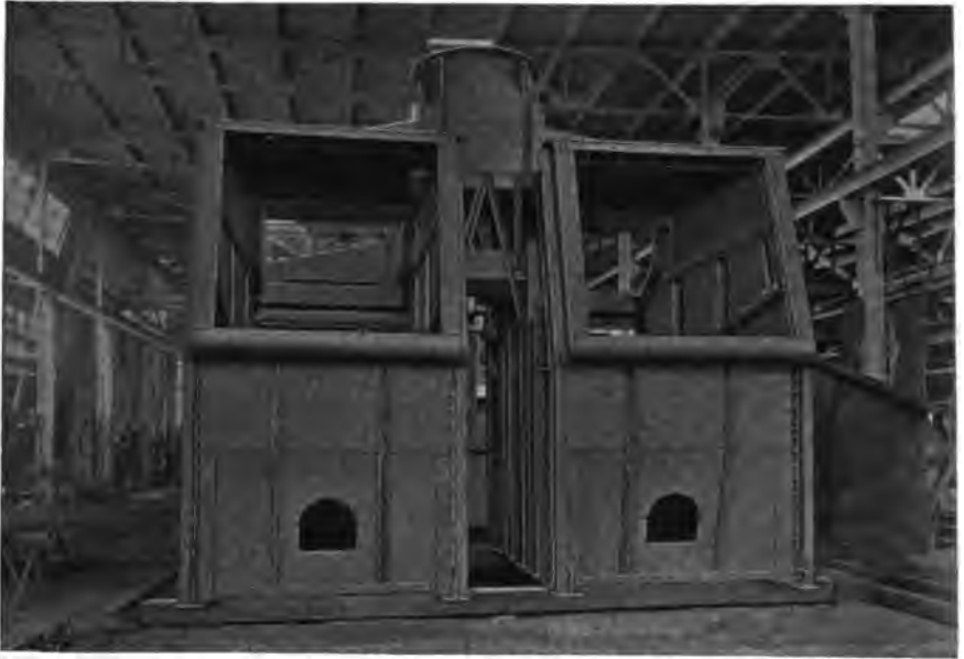
Front View of Marine Casings for a Battery of Two Heine Cross Drum Marine Boilers.
