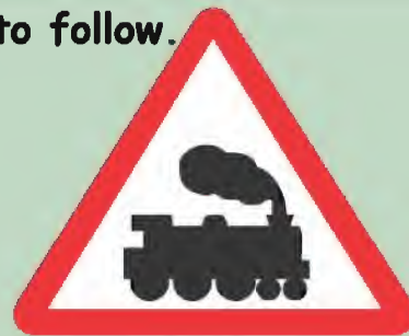
Unguarded Rail Crossing
