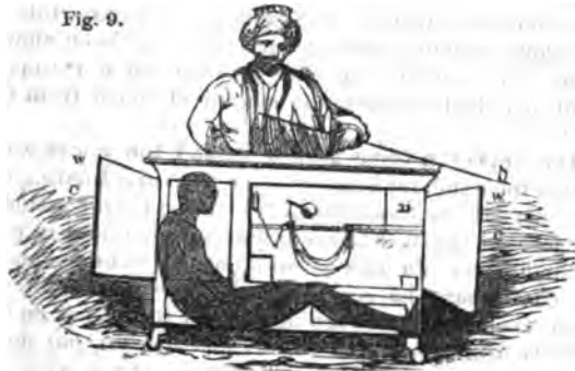
A front elevation, showing the concealed player in his second position, when the door is closed and A C O open.
