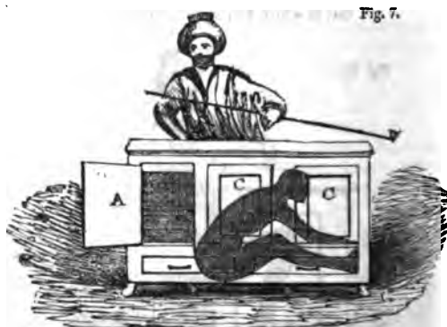
An elevation of the front of the chest, showing the concealed player in his first position when the door A is opened.
