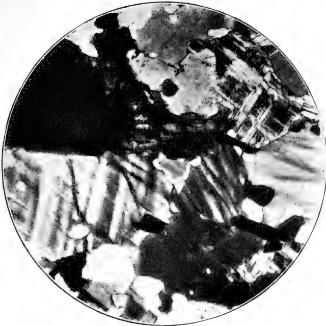
PLATE XIX. FIGURE 1. PHOTOMICROGRAPH OF THE CAMPBELL-COWETA-MERIWETHER COUNTIES' MEDIUM BLUE-GRAY GRANITE. TWO MILES NORTH OF FAIRBURN, CAMPBELL COUNTY, GEORGIA. CROSSED NICOLS X74.
