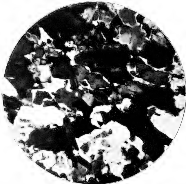
PLATE XXII. FIGURE 2. PHOTOMICROGRAPH OF A FINE-GRAINED DARK-BLUE BIOTITE GRANITE FROM A DIKE FORTY FEET WIDE, CUTTING THE PORPHYRITIC GRANITE-GNEISS, NEAR CAMAK, WARREN COUNTY GEORGIA. CROSSED NICOLS \times 74 .
