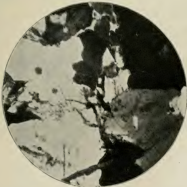
PLATE XVIII. FIGURE 2. PHOTOMICROGRAPH OF THE ECHOL'S MILL LIGHT-GRAY GRANITE. ELEVEN MILES NORTHEAST OF LEXINGTON, OGLETHORPE COUNTY, GEORGIA. CROSSED NICOLS x74.
