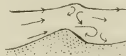
FIG. 2. SCHEME OF VORTICAL MOVEMENTS ABOUT THE CREST OF A CURRENT MARK. THE SHADED SLOPE SHOWS THE AREA ON WHICH THE PARTICLES OF MICA HAVE COME TO REST BENEATH THE NODE JUST IN ADVANCE OF THE CREST. (AFTER SKETCH BY JAGGAR.)
