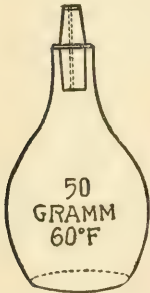
FIG. 19.—Drawing showing the type of pycnometer generally used in determining the specific gravity of soil. The ground-glass stopper is perforated.
