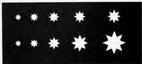
STAR SYMBOLS illustrate arithmetic (top) and geometric (bottom) area increases. Upper symbols grow by a constant increment and lower ones increase by constant ratio (1.2:1).
