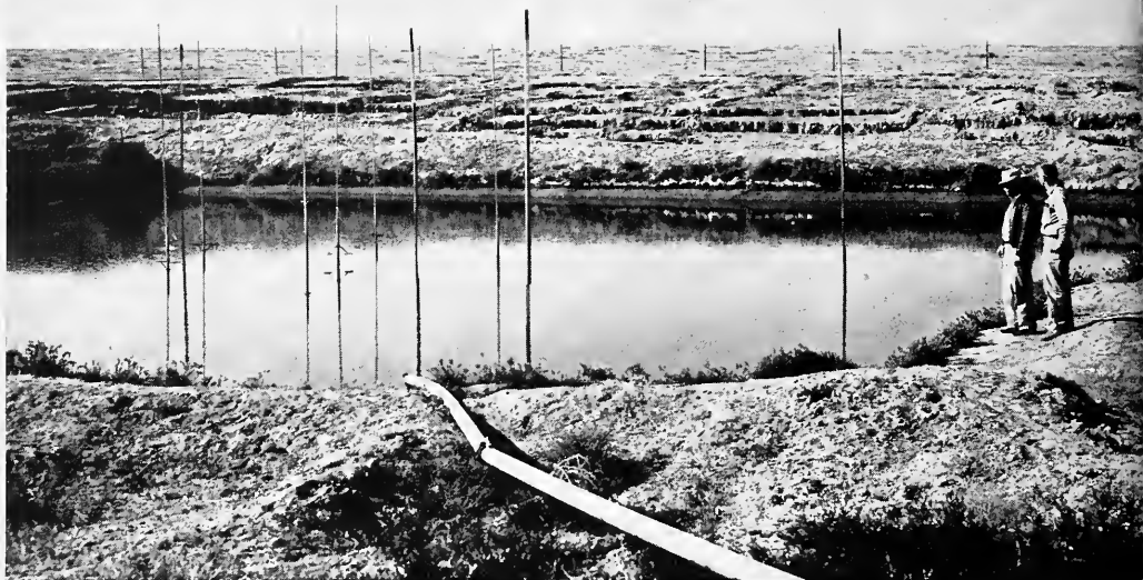
HYDROCOMPACTION test plot shows ten-foot drop after previously level land was subjected to 17 months of flooding.
