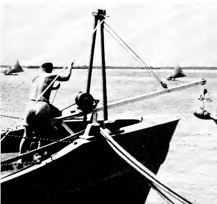
SOUNDING WEIGHT and a current meter, attached to cable reel on suspension boom, are lowered for depth readings.
