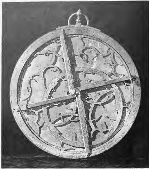
ASTROLABE, early navigation instrument to determine time and latitude by star sighting, was made in 1581. It antedates the Gregorian reforms and shows the equinox on March 10.
