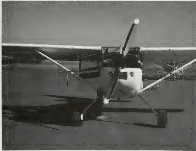
Yagi antenna mounting system on aircraft.
