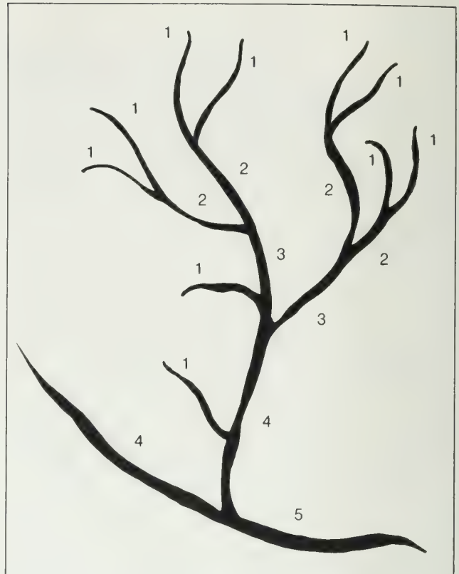
Figure 1. Stream order by A.N. Strahler (1952).
