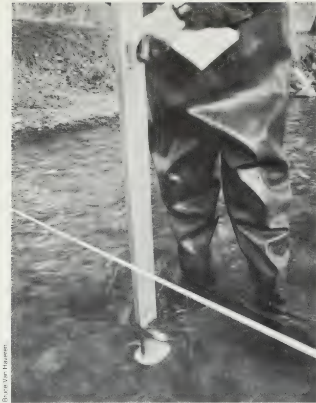
Figure 7. A velocity-head rod for measuring stream velocity.
