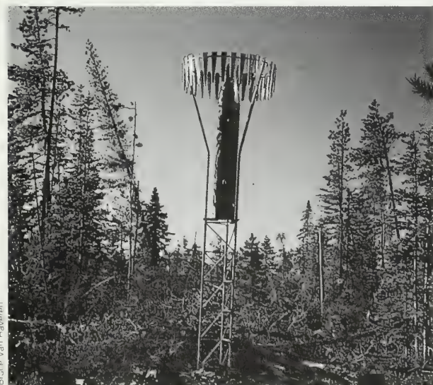
Figure 1. A precipitation storage gage with an "alter shield" at an ideal gage site in a forest clearing.
