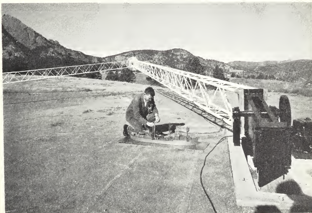
The complex antenna system of the U.S.N.S. Eltanin was evaluated using a 60:1 scale model ship and the NBS antenna test range. The Eltanin is a National Science Foundation ship designed for geophysical research in the Antarctic. (See p. 145.)
