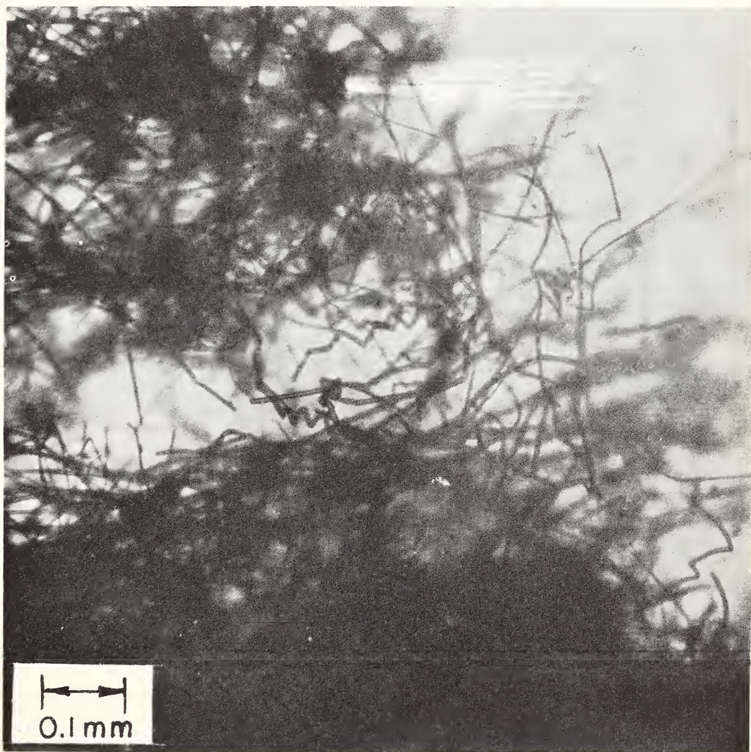
Fibrous silica grown in a study of the structural relationship of the amorphous forms of silica to each other and to the crystalline forms. The exact nature of this form of silica is now being investigated. (See p. 94.)
