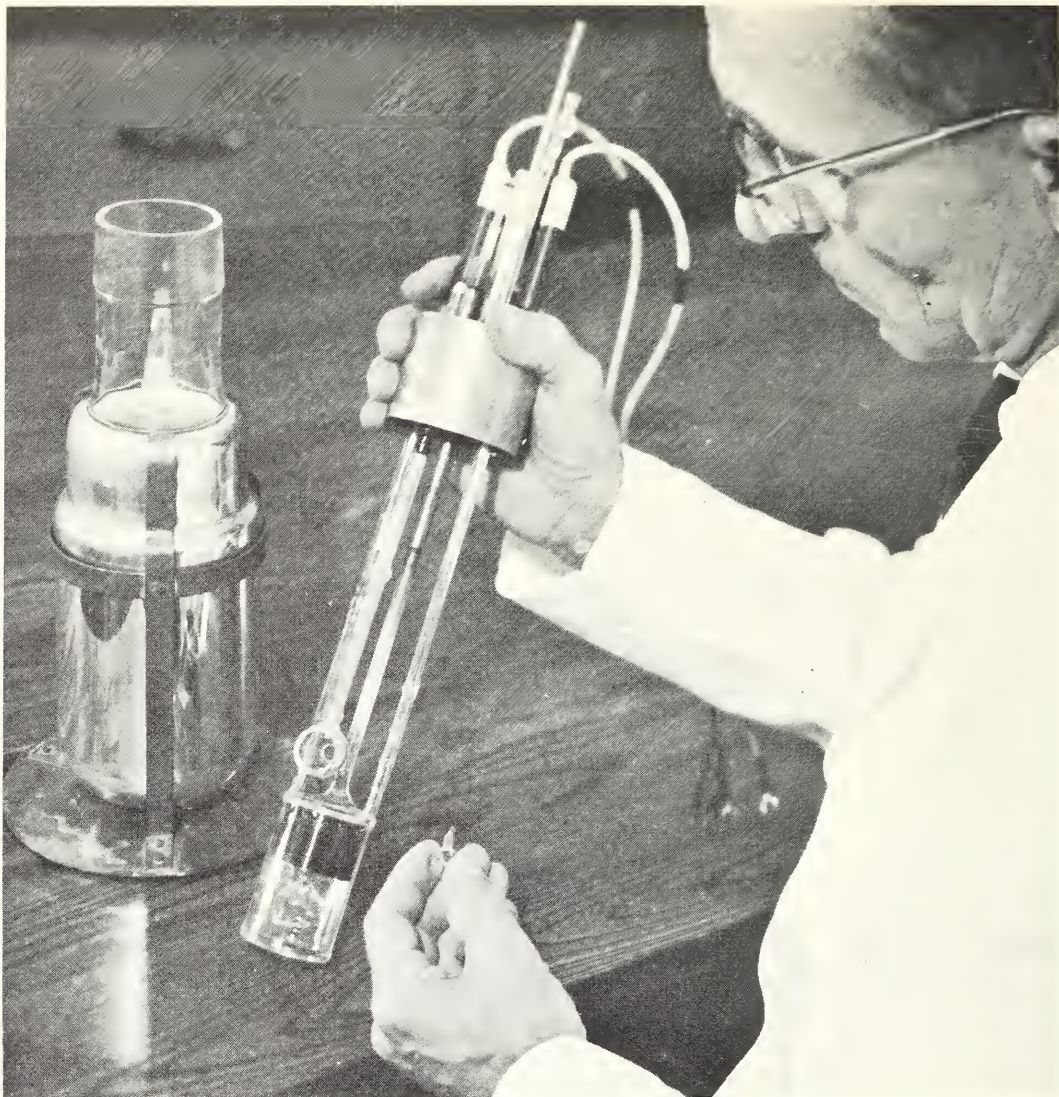
Solution calorimeter used in precise measurements of heats of solution and liquid phase reactions. Recent studies have concentrated on beryllium compounds. (See p. 85.)
