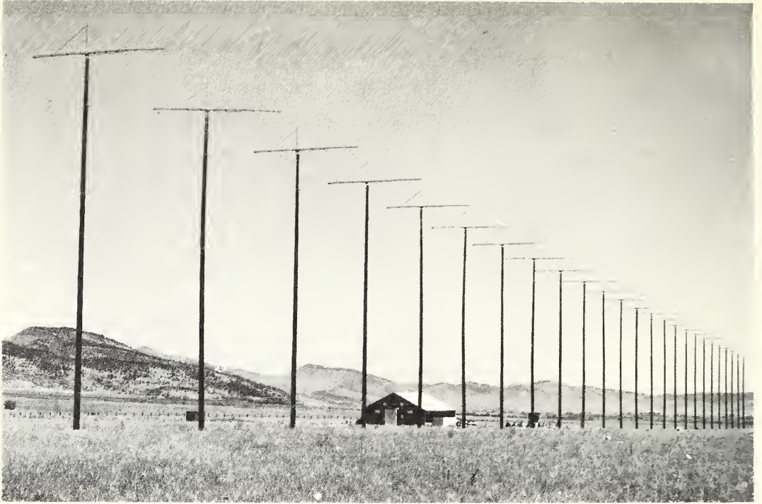
Array of 25 antennas used to study the effects of ionospheric irregularities on radio signals propagated over long distances. (See p. 144.)
