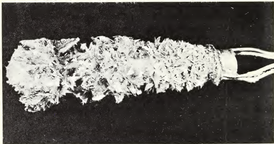
Deposition of silver on silver single crystal after exposure to molten sodium chloride in a silver crucible for 15 hours. Such studies have shed much light on electrolytic processes. (See p. 43.)
