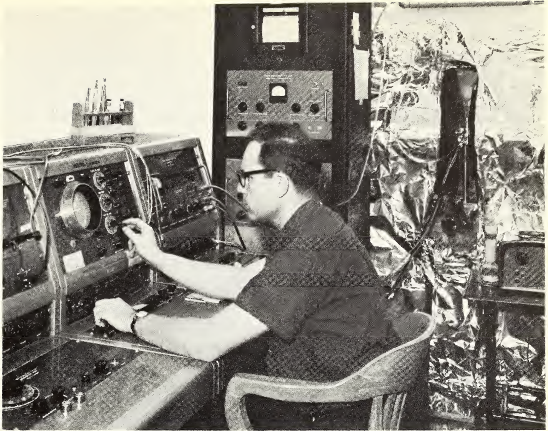
Apparatus for obtaining nuclear magnetic spectra, which reveal important information on the local electronic environment of nuclei in complex molecules, on the sites of specific chemical reactivity, and on the pathways for communicating electronic effects within these molecules (page 82).
