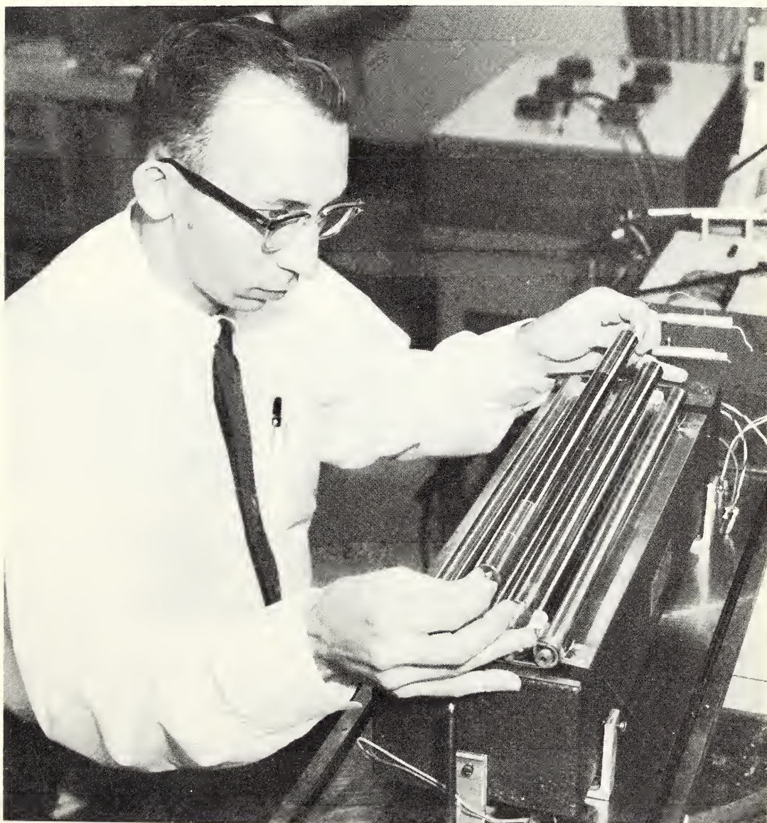
Assembling the gage blocks used to form the NBS computable cross capacitor. The capacitor was used to re-evaluate fundamental unit of resistance in terms of the prototype standards of length and time (page 36).
