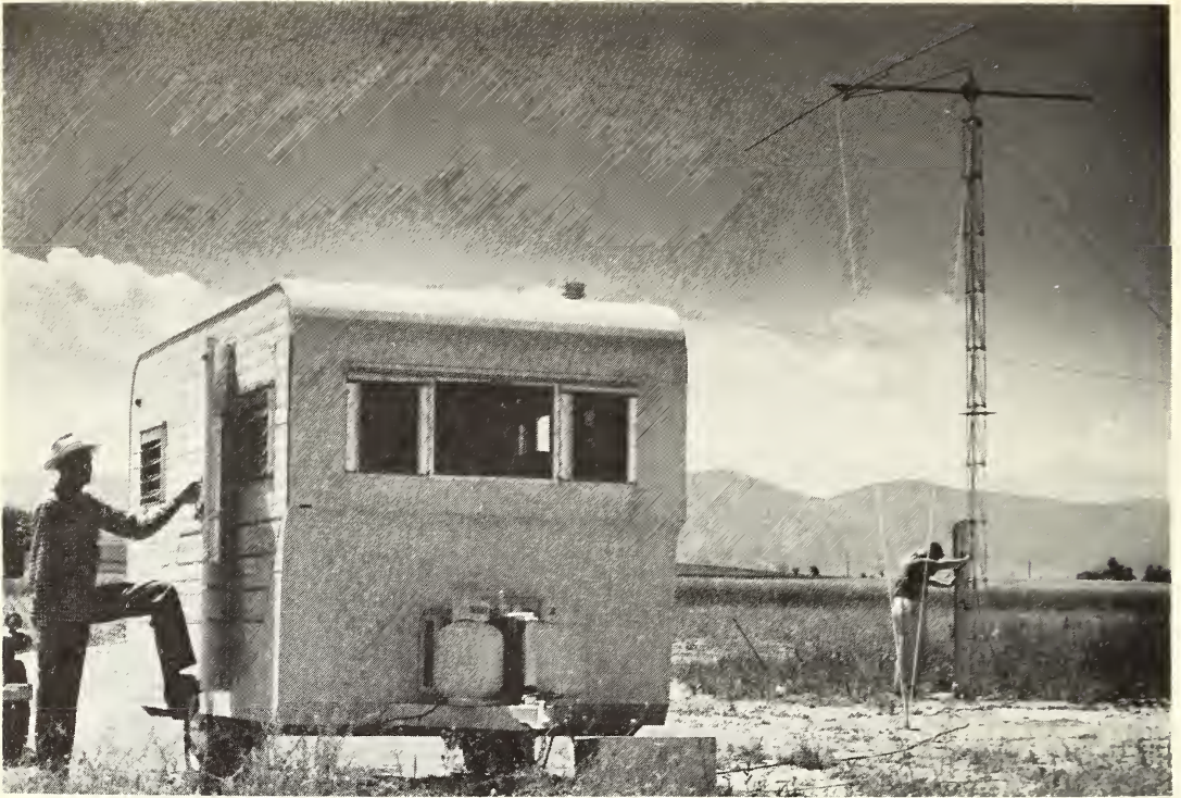
A mobile satellite observing station, in conjunction with permanent facilities at Table Mesa, is being used to study ionospheric irregularities and their effect on the reception of satellite signals (page 141).
