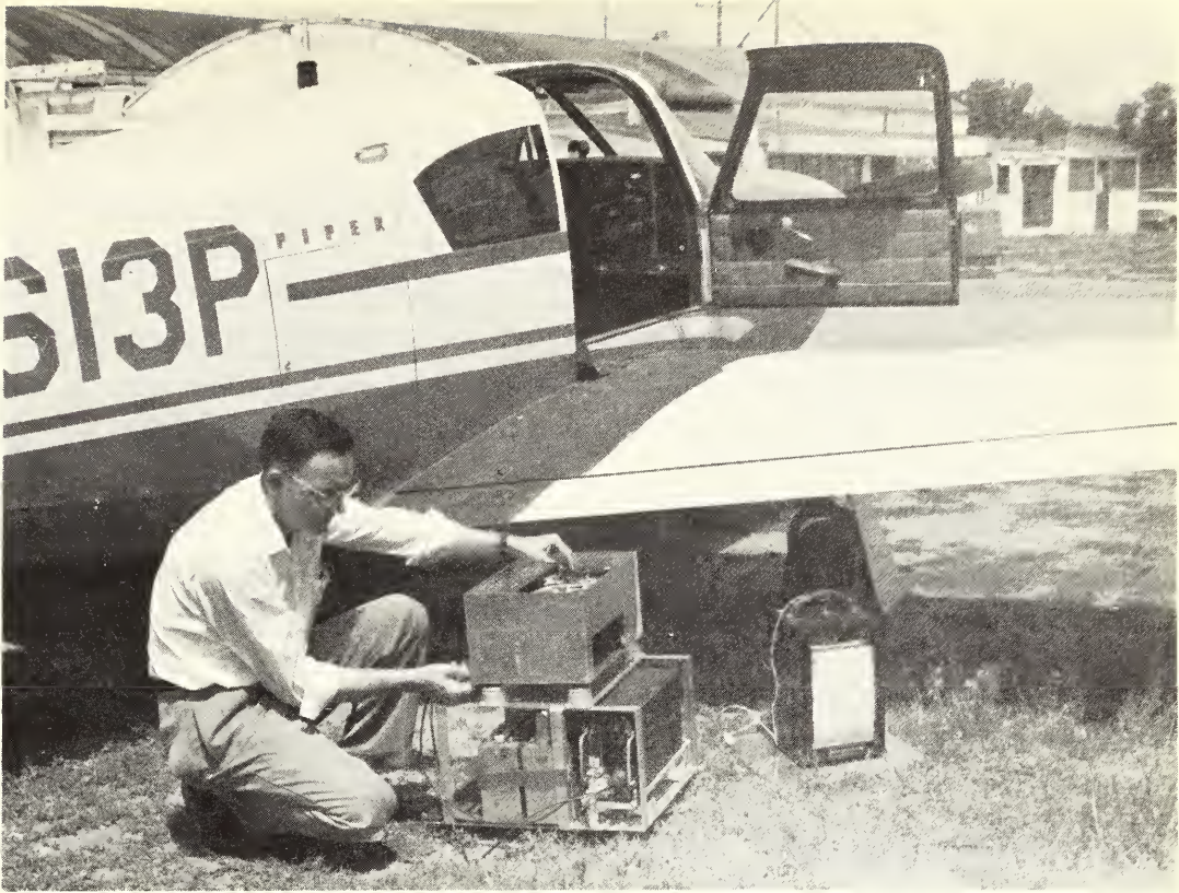
Airborne refractometer equipment used in studying the effects of atmospheric inhomogeneities and turbulence on missile radioguidance systems using microwaves (page 130).
