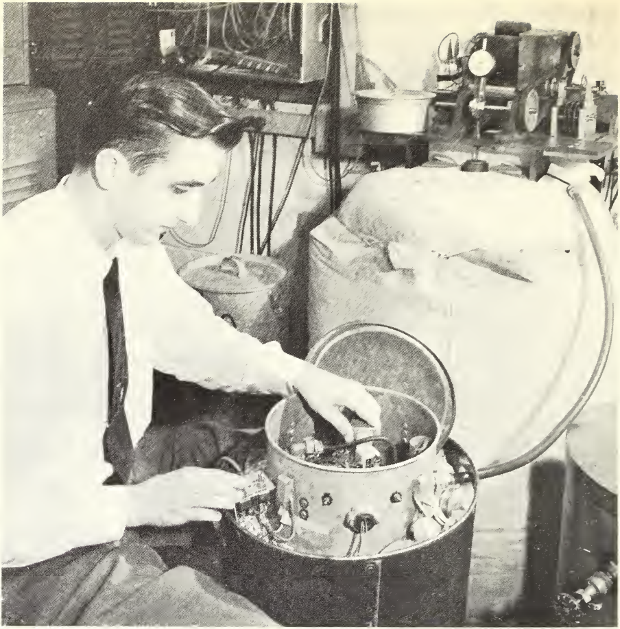
Calibrating an infrasonic microphone (front, connected by a hose to the calibrating barrel) used to study naturally occurring infrasonic sound waves in the atmosphere (page 29).
