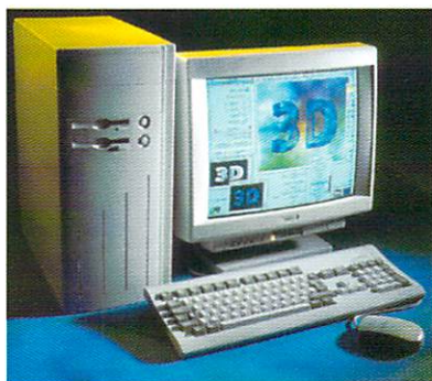
Micronik's custom tower snugly takes all your A1200 bits, adds Zorro II slots and more
