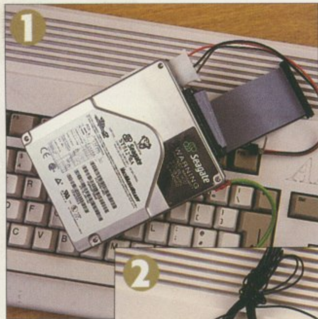
1 The slimline Seagate 1Gb hard drive is a perfect size for the A1200
