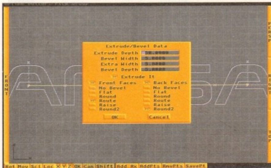
Imagine's new Spline editor allows you to work with PostScript fonts and other 2D objects and extrude them
