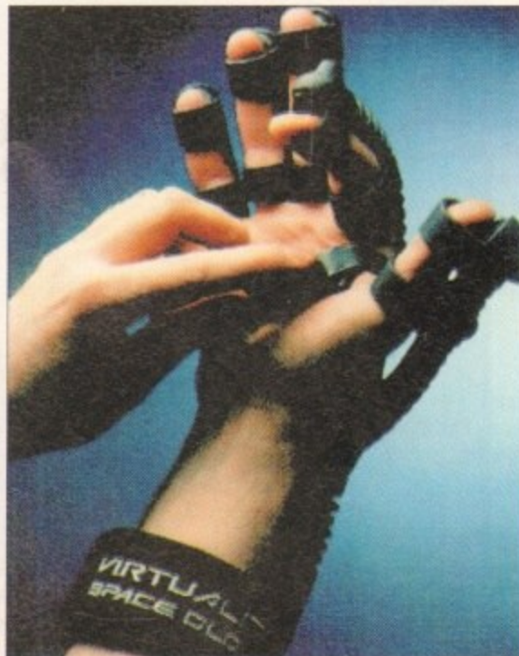
Touch Glove allows users to feel virtual reality objects
