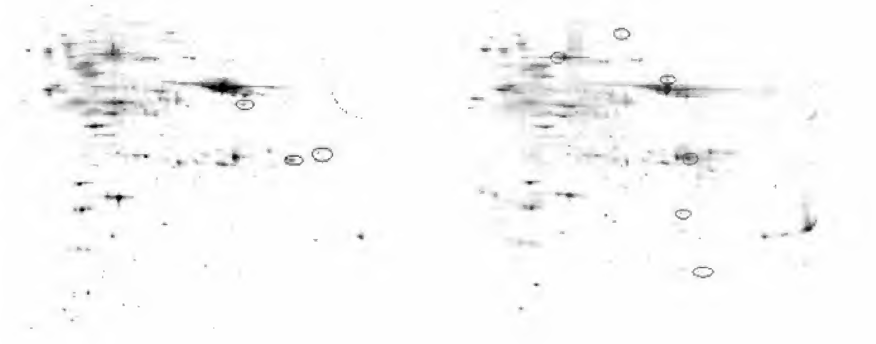
Fig. 23.3 Two-dimensional gels from root plasma membrane of seedlings grown in the absence ( left ) or presence ( right ) of 100 \mu\text{m Cd}^{2+} . Protein spots which differ in the two preparations are marked
