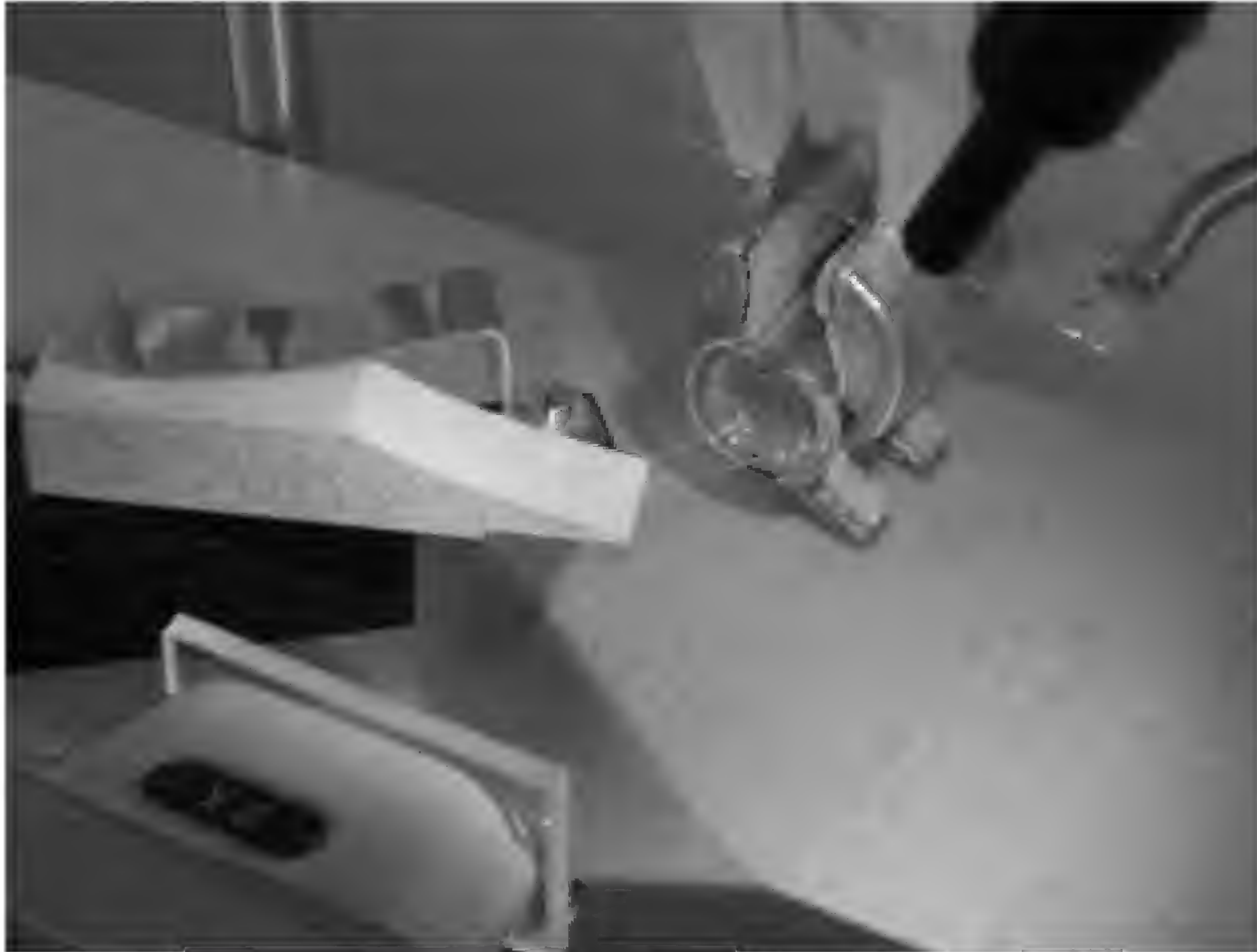
Fig. 17.1 Transfer platform for small samples fixed in front of the quartz fiber balance housing
