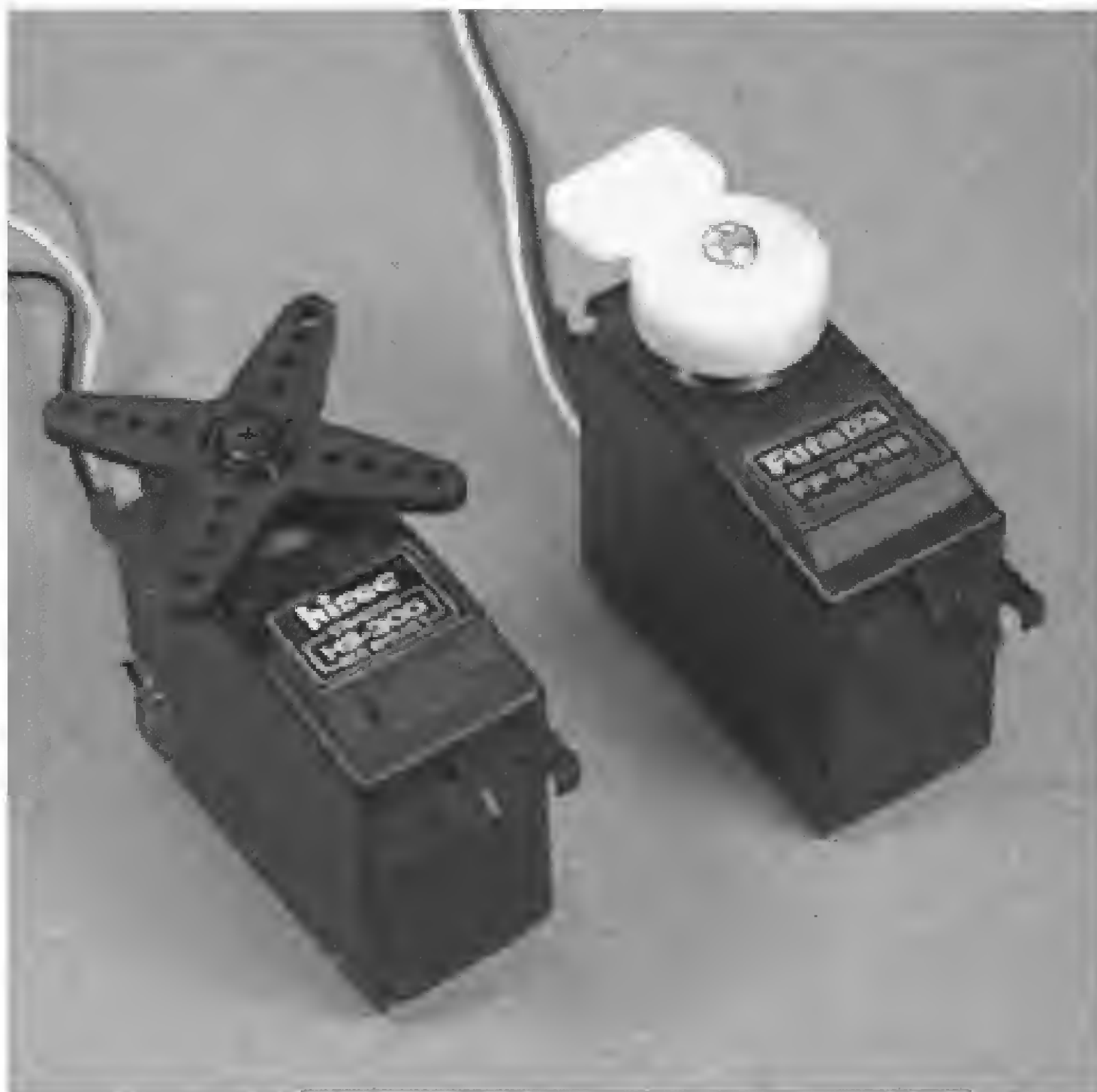
Figure 13.1 Picture of hobby 4- to 6-v (42-oz torque) servomotors.
