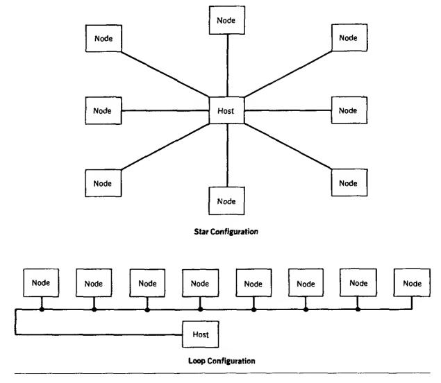
FIGURE 9.1 Communication Configurations
