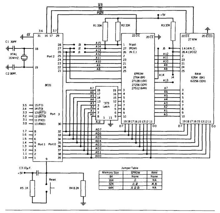
FIGURE 7.1 8031 Microcontroller with External ROM and RAM
