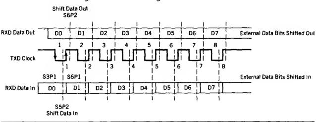
FIGURE 2.14 Shift Register Mode 0 Timing
