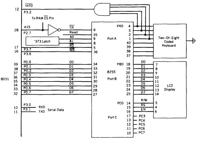
FIGURE 8.14 A Multi-Tasking Circuit Using Memory-mapped I/O
