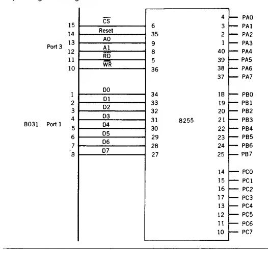
FIGURE 7.3 Expanding I/O Using 8031 Ports
