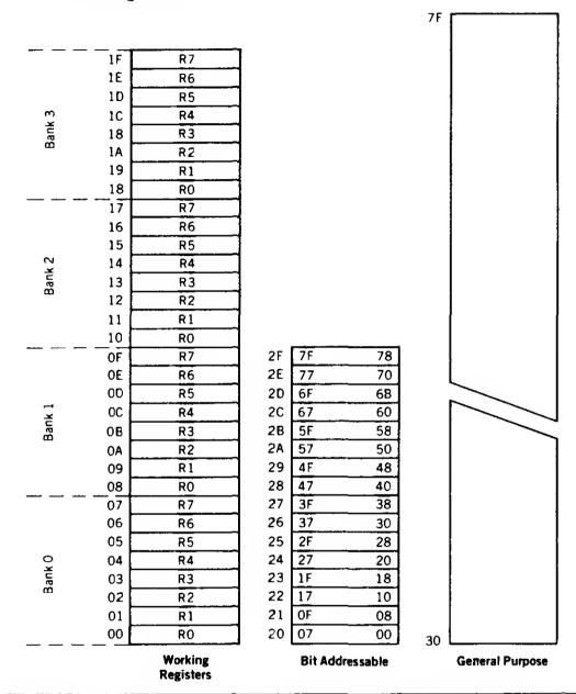
Note: Byte addresses are shown to the left; bit addresses registers are shown inside a location.
