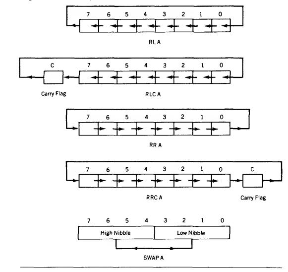
FIGURE 4.2 Register A Rotate Operations
