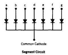
Figure 8.7. A segment will be lit *only if* the segment line is brought high *and* the common cathode is brought low.
