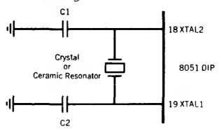
**Crystal or Ceramic Resonator Oscillator Circuit**
