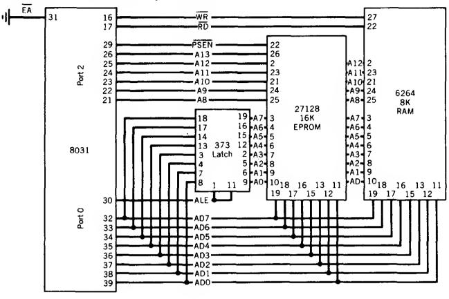
FIGURE 2.8 External Memory Connections
