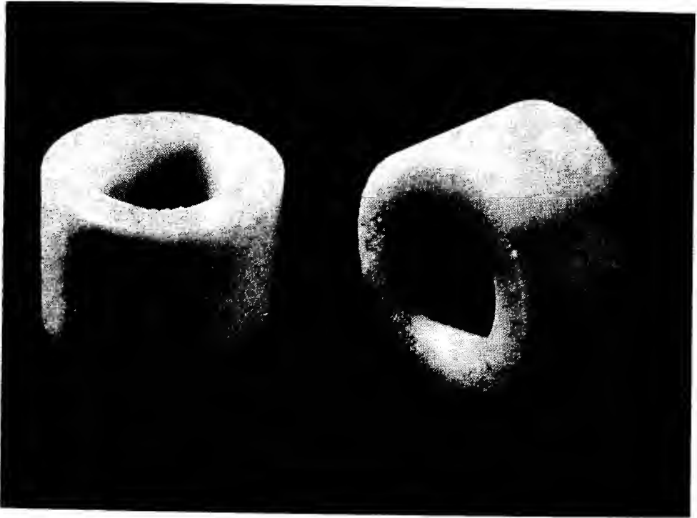
FIG. 142. Rings of sodium chloride or sodium hydrogen carbonate for making rigid sheaths (Courtesy Dr. L. Deffet, Sterrebeck, Belgium).
