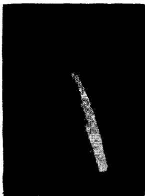
FIG. 129. Flame from dynamite having a low nitroglycerine content (Gelatine-Dynamite). Duration 1.25 millisecc (according to Bichel [16]).
